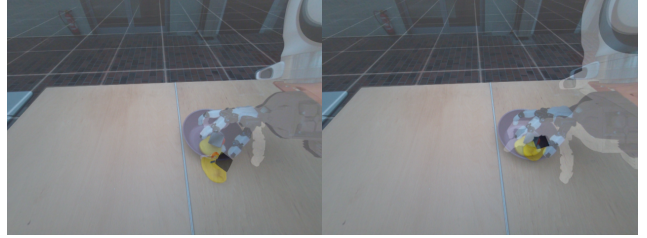
Figure 5. Terminal-frame alignment of the object with the real recording. (Left) Open-loop dynamic replay drifts from the recorded duck. (Right) Our residual policy stays aligned.
